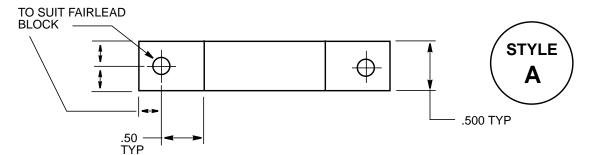
APPLY TAPE TO PROFILE OF OUTER FAIRLEAD BLOCK TYPICAL AS SHOWN - ADHESIVE SIDE AGAINST BLOCK MATERIAL:
