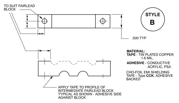
NOTE: THIS IS A TYPICAL PROFILE FOR APPLICATION OF TAPE - NOT A PART
