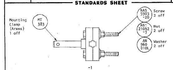
Replace existing commercial screw, nut and lockwasher combination on MT383 mounting clamp (Arens) with the hardware shown on drawing.
