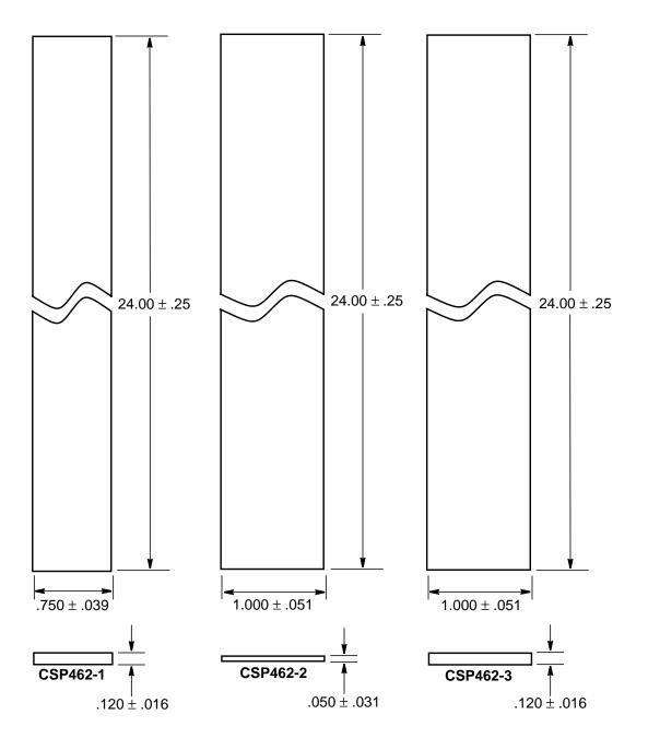
MATERIAL: MIL-R-25988 Type II, Class 1, Grade 60, Fluorosilicone Rubber
