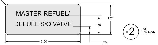
DIRECT SCREEN PRINT ON WHITE, SELF-ADHESIVE VINYL FILM, DSC85-2A PER PPS 22.06 -- OR-- DSC85-6B PER PPS 22.12 CHARACTERS, 12 POINT, UNIVERS 67, COLOUR BLACK (FED STD 595-27038)
