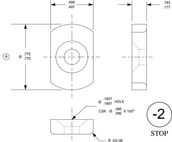
MATERIAL: MIL-S-18729 or MIL-S-6758, 4130 COND 'N', .187 THICK FINISH: E1 or CADMIUM PLATE PER QQ-P-416, TYPE II, CLASS 2
