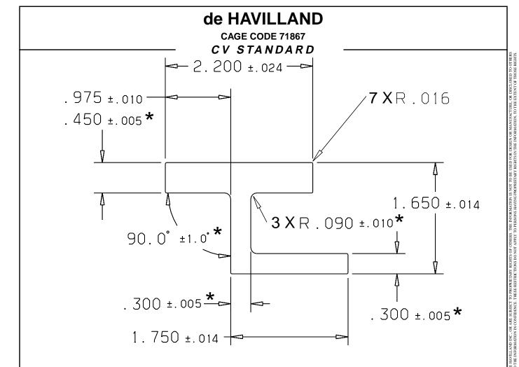
MAT'L AL ALLOY 7150-T77511 AMS 4345 UNLESS OTHERWISE STATED FED. STD #245 TOLERANCES APPLY MIN. LENGTH 30 FT.
