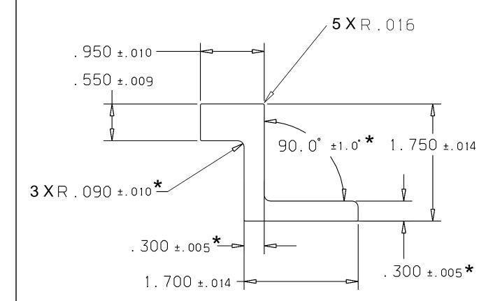
MAT'L AL ALLOY 7075-T76511 QQ-A-200/15 UNLESS OTHERWISE STATED FED. STD #245 TOLERANCES APPLY MIN. LENGTH 30 FT.
