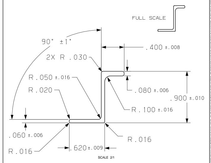
MATERIAL: ALUMINUM ALLOY 7150-T6511 SPECIFICATION: QQ-A-200/11 UNLESS OTHERWISE STATED FED. STD #245 TOLERANCES APPLY
