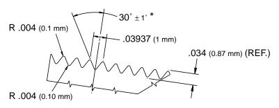
VIEW ON ARROW "P" (SERRATION DETAILS - SEE ALSO NOTE 4) (SCALE 5:1)
