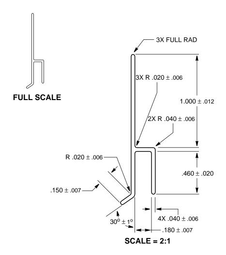
MATERIAL: ALUMINUM ALLOY 2024-T3511 SPECIFICATION: QQ-A-200/3 FED. STD #245 TOLERANCES APPLY
