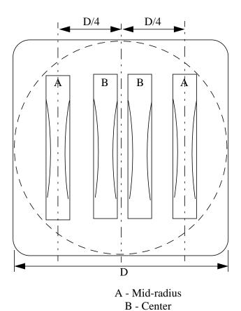
Fig. 1 Location of transverse tensile specimens.
