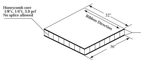
2 plies of product to be qualified with warp direction parallel to ribbon direction. Place warp face against the core.
