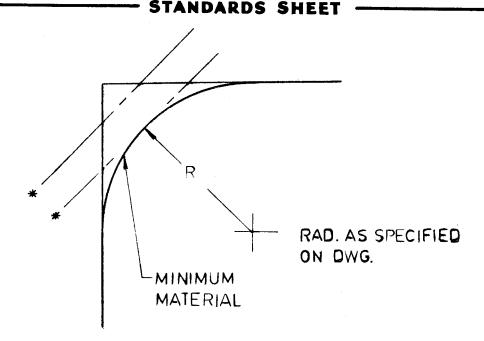
The purpose of this standard is to save manufacturing cost on sheet metal details and extruded parts and is applicable to outside profiles only.
