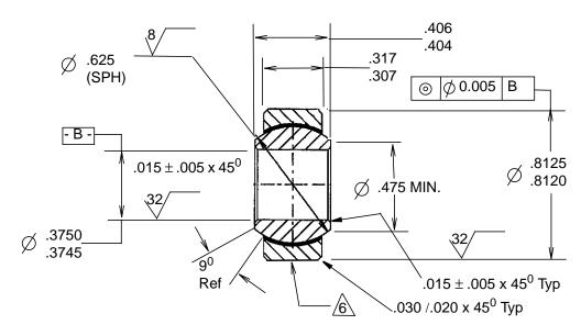
**★ DSC 569 BEARING IS DIMENSIONALLY EQUIVALENT TO MS14104, ALSO BEARING SHALL MEET THE AS-81820 REV. A REQUIREMENTS EXCEPT AS FOLLOWS:**
