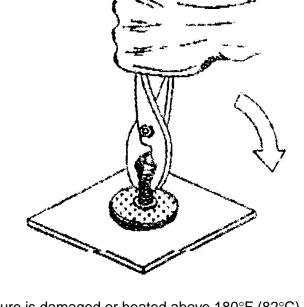
or scratch the structure; if the structure is damaged or heated above 180°F (82°C), refer to Liaison Engineering for disposition.
