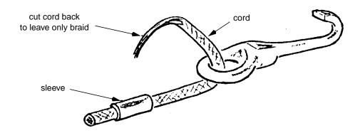
Step 2. Using the installation tool, draw the end of the cord back through the sleeve as shown below.
