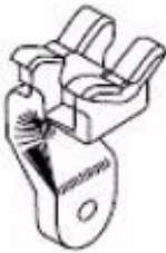
B0816026 / MS3340 / LHM Sxxx Riveted transverse bulkhead type single harness tie mount
