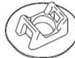
CLICK BOND CB3019 Adhesive bonded cradle type single harness tie mount
