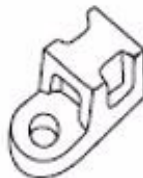
B0816006 / TA1xxx Riveted miniature type single harness tie mount
