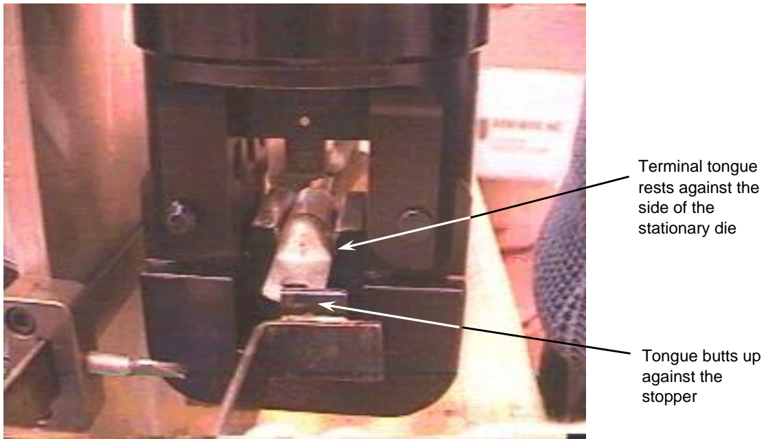
Figure 5. Positioning of Copalum Terminal Lug in Crimping Tool
