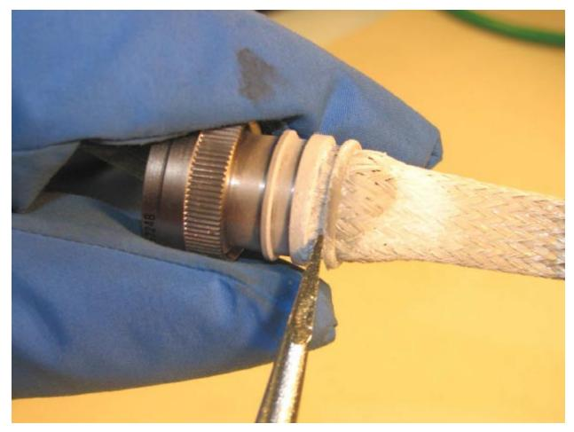
Step 2. Position the cutting blades of the removal tool (ref. paragraph 4.2.1) squarely over the Tinel-Lock ring.
