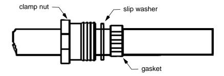
Step 2. Strip the outer jacket from the end of the twinaxial cable according to PPS 9.24 to expose 0.406" of the braided shield as shown below.
