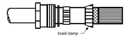
Step 5. Form the combed braid back over the braid clamp and trim flush with the end of the braid clamp/end of the outer jacket as shown below.
