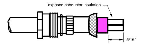
Step 7. For each of the conductors, trim back the conductor insulation 1/8" according to PPS 9.24 as shown below.
