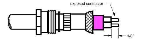
Step 8. Assemble the twinax connector bushing, insulator and contacts over the conductors as shown below.
