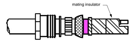
Step 11. Slide the gasket, slip washer and clamp nut against the braid clamp and the connector body over the mated insulators in order to thread the clamp nut into the connector body. Tighten the clamp nut to 30 in. lbs. according to PPS 14.01, such that the vee gasket is split by braid clamp.
