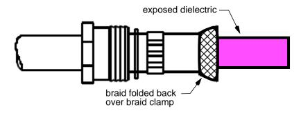
Step 6. Trim back the dielectric 5/16" from the end of the twinaxial cable end according to PPS 9.24 as shown below.
