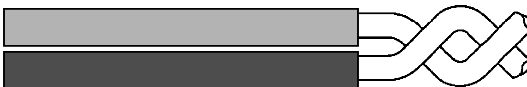
FIGURE 2 - TWISTING OF THERMOCOUPLE ENDS
