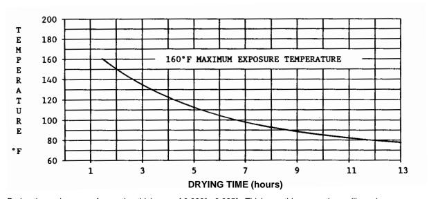
Drying times shown are for coating thickness of 0.020" - 0.025". Thicker or thinner coatings will require proportionally longer or shorter drying times.
