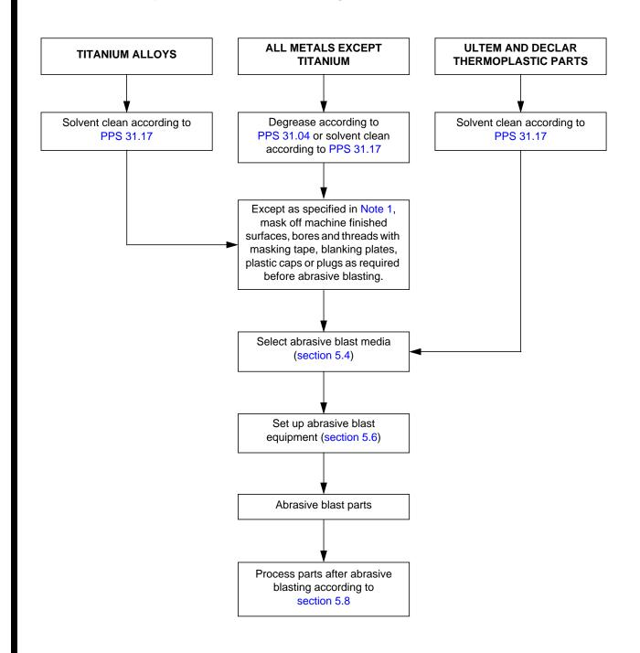
Notes 1. Before abrasive cleaning with fine glass bead or fine aluminum oxide (grit size 180 maximum), only surfaces having a surface finish finer than 32 RMS require masking.
