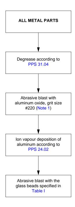
Notes 1. The maximum time allowed between abrasive blasting using aluminum oxide grit and the ion vapour deposition of aluminum is 4 hours.
