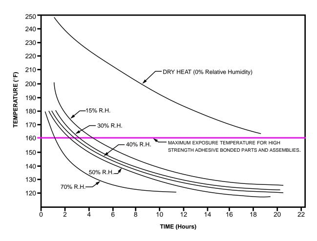
Note 1 Allow a minimum drying time as specified in paragraph 5.2.4.1 before curing at higher temperatures. Note 2. If the above heat cure chart conflicts with the primer manufacturer's technical data sheet, follow the manufacturer's instructions.
