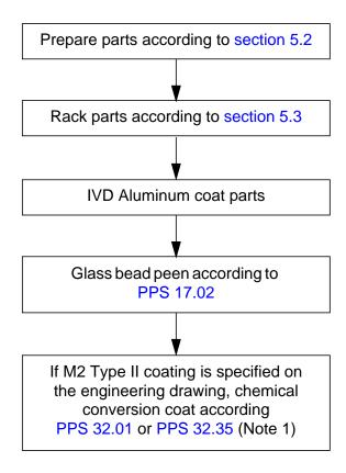
Note 1. Chemical conversion coat according to PPS 32.35 if the engineering drawing specifies a protective treatment code C10 (i.e., where low electrical resistance is required).
